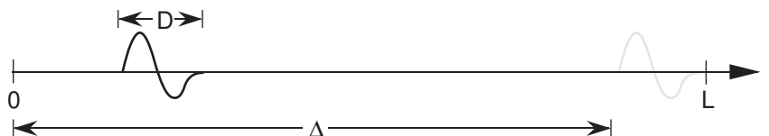
Figure 5.14: Despite uncertainties in the signal's delay \Delta , the signal is assumed to lie entirely within the observation interval. Hence the signal's duration D , the duration L of the observation interval, and the maximum expected delay are assumed to be related by \max \Delta + D - 1 < L . The figure shows a signal falling properly within the allowed window and a grey one falling just outside.
